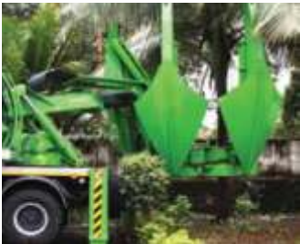
360° slew mechanism Enhances accessibility to the tree by allowing the vehicle to be parked in any position, reducing the need of moving the truck back and forth to come to the required position, thereby improving fuel efficiency.
