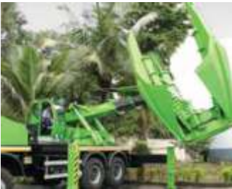
Hydraulic telescopic boom Permits access to trees located at a distance, where the vehicle might not be able to reach due to obstacles.
