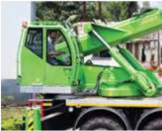
Operator console cabin Enhances the operator ergonomics, which is essential to minimize the damage that might be caused while uprooting the tree.
