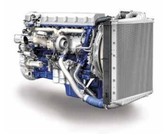
The D13A460 is a 460 hp 12.8-litre in-line, six-cylinder diesel engine equipped with an overhead camshaft, four valves per cylinder and unit injectors. The engine meets the EU exhaust emissions requirements according to the Euro 4 standards.
