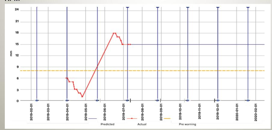
Predictive maintenance monitors the life of truck components to enable proactive planning and timely repairs.
