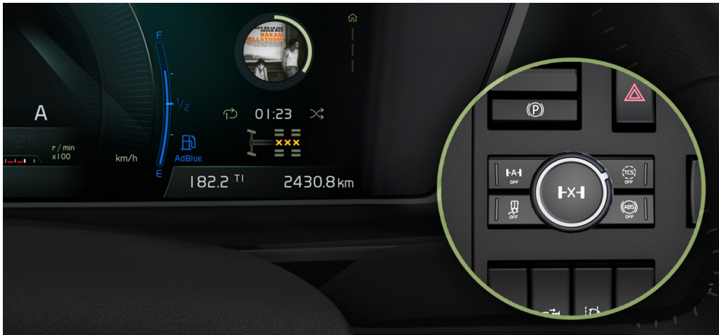
Traction Control knob & display
